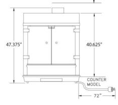
Unit shown with dome in back counter orientation.
